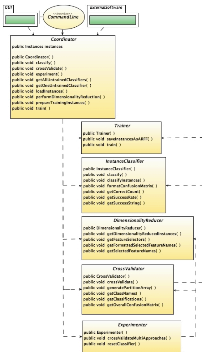
Figure 1. Structure of ACE's main processing classes. The Coordinator class provides an exclusive interface through which ACE's main functionality can be accessed. Arrows indicate interactions between classes. All public methods are listed, but parameters are omitted from method declarations to save space.
